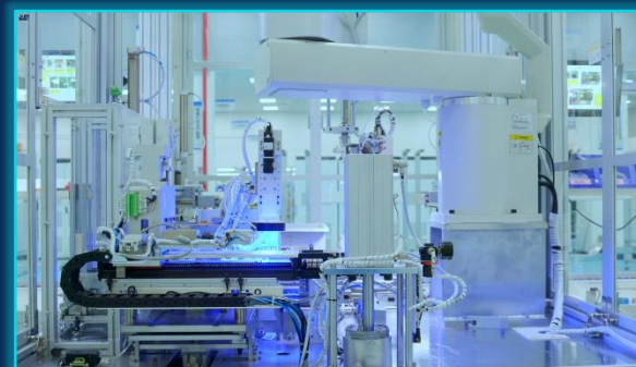
Automatic application of silicone grease
