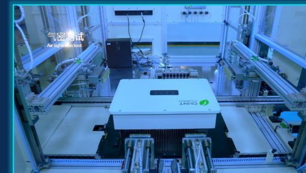
Fully automatic airtightness test
